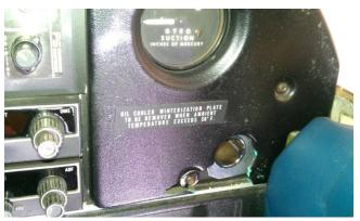
**55044** has completed a 50 hour, and the electric trim – always a problem piece of equipment – has been completely disconnected. In addition, the "cigarette lighter" (car charger?) has been replaced – careful use should keep the wires from being broken again; please attach any electronics carefully with a minimum of twisting if you can.
