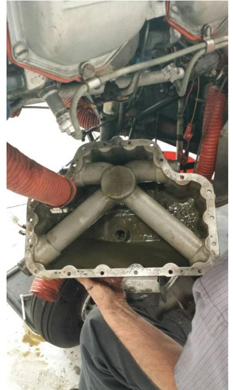
The oil pan sits below the cylinders, ready to supply the system with oil for cooling and lubrication.
