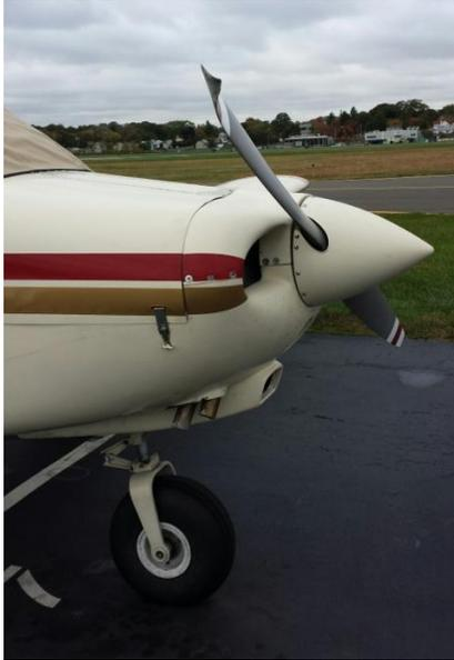
A Piper Tomahawk at the airport had a prop strike (veered off runway during a crosswind landing and struck – barely – a runway light) and had to have its engine torn down to inspect for damage. Note only one blade bent, but even so, the plane was unable to take off. Enjoy these photos of the inner workings of a Lycoming engine!
